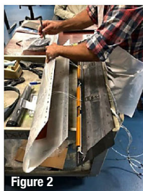
Figure 2 (left): Installation of leading edge and thermal-mechanical expulsion de-icing system assembly. Figure 3 (right): Snapshots taken from recording of icing tunnel test showing complete de-icing on coated leading edge (bottom) and no de-icing on uncoated leading edge (top), at power consumption level 70% lower than that of the nominal power needed for a regular functional uncoated de-icing system.
