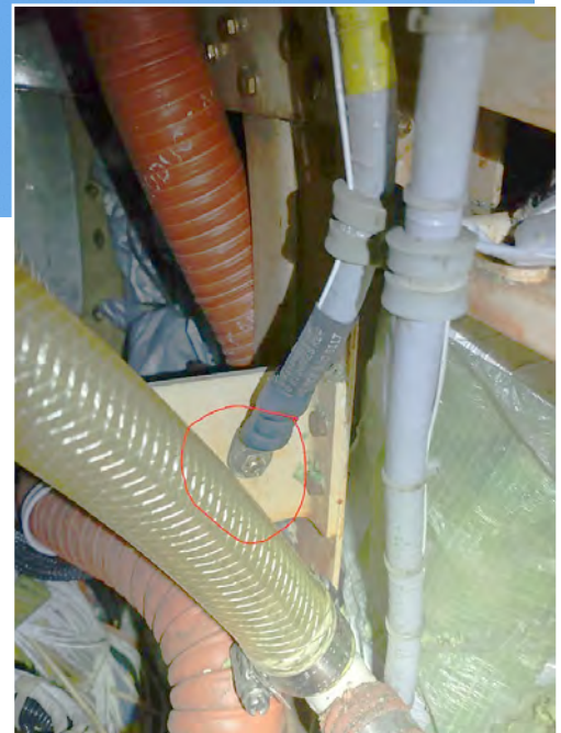
Below: Battery ground wire stud back side showing 2 nuts installed.
