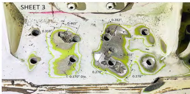
Below: Close up of worst area of corrosion in center section.
