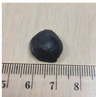
Airbus. Piece of FOD found in fuel tank.
