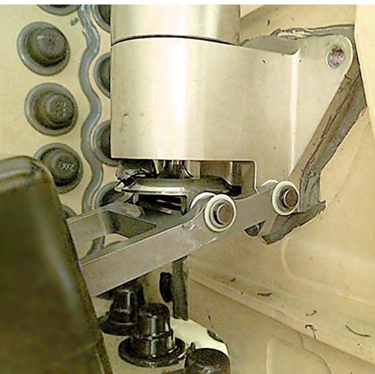
Airbus. Piece of FOD found in shut-off valve.
