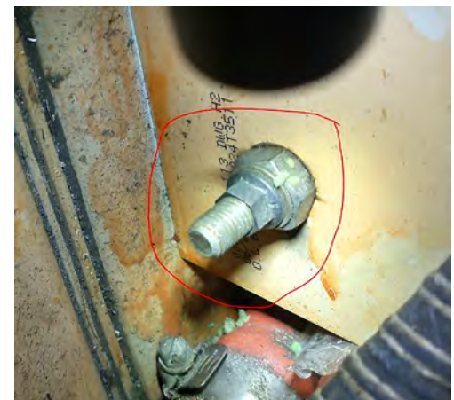
Below: Battery ground wire stud back side showing 2 nuts installed.
