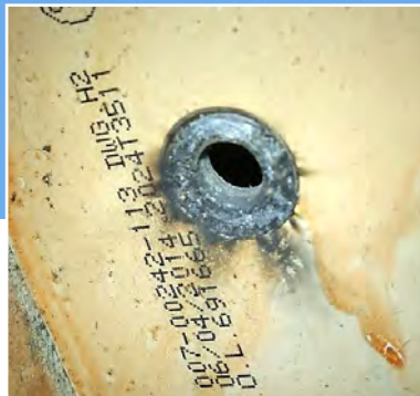
Right: Back side frame showing corrosion and arcing. Far right: Battery ground wire front view.
