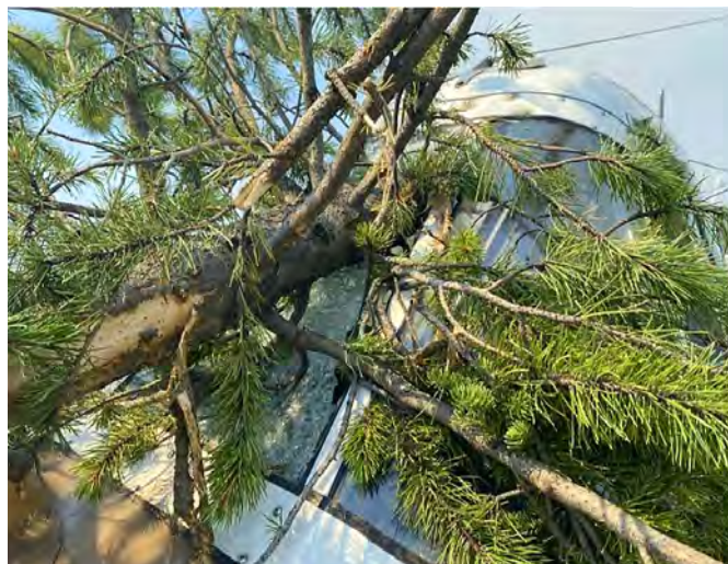
Tree protruding through the front windscreen and into the cockpit of the occurrence aircraft after its collision.
