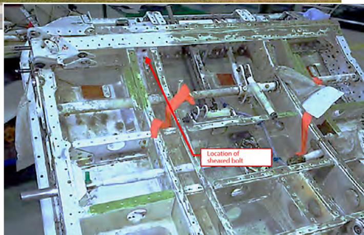
Left: Broken bolt location back side.
