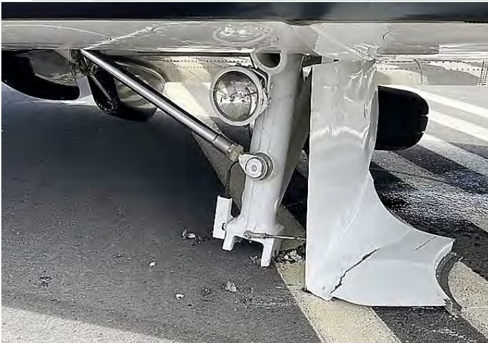
Left: Fractured gear impacting the runway.
