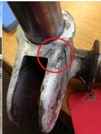
Piper PA-28. Right: Inner radius of stub axle lug.
