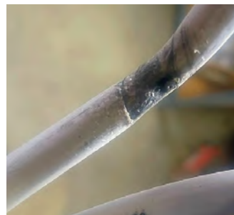
Above: a Beech 1900D Far left: Location of concern above logo light, internal of stabilizer. Left: The melted deice line.
