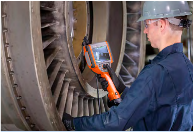
The Intelligent Borescope provides consistent and fast data collection.
