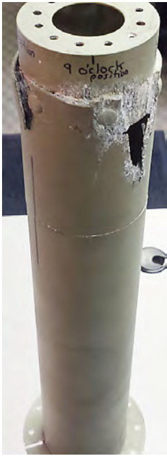
Aircraft: a Cessna 208. Left: Cessna, Elevator torque tube with excessive corrosion at end cap.
