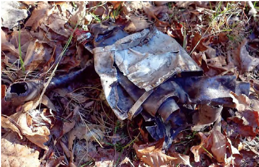
Left: The wreckage of the muffler from the CO poisoning accident.
