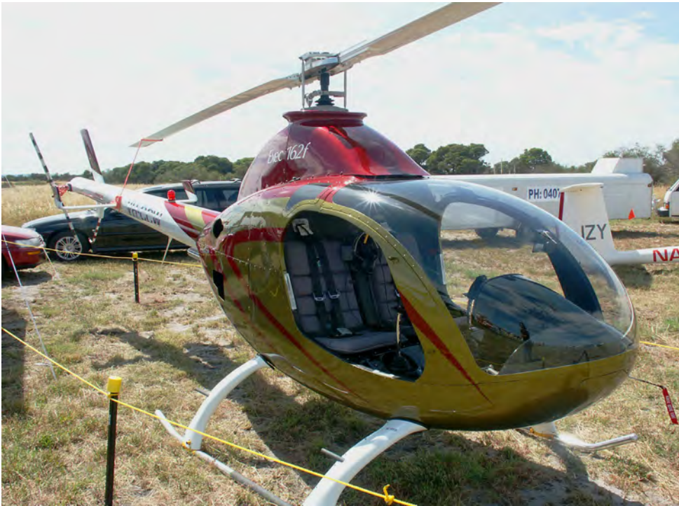
Left: Unlike most U.S.-designed helicopters, the main rotor on the Exec 162F rotates clockwise.
