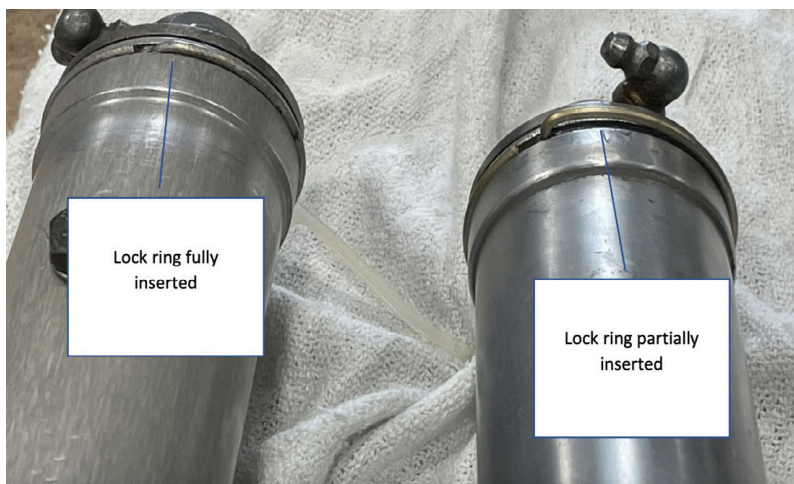
Right: Figure 8. Exemplar horizontal stabilizer actuators and lock rings.
