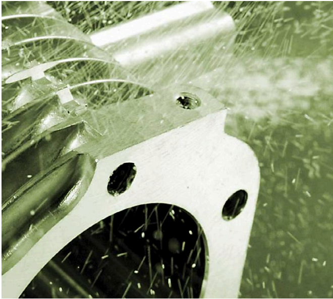
Silica sand used in abrasive blasting typically fractures into fine particles and becomes airborne.
