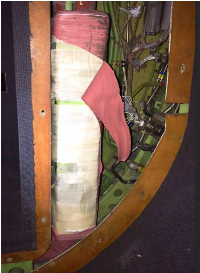
Left: Muffler as installed, adjacent to the hydraulic filter manifold, outer insulation wrapping damage is evident. Above: A Learjet 45
