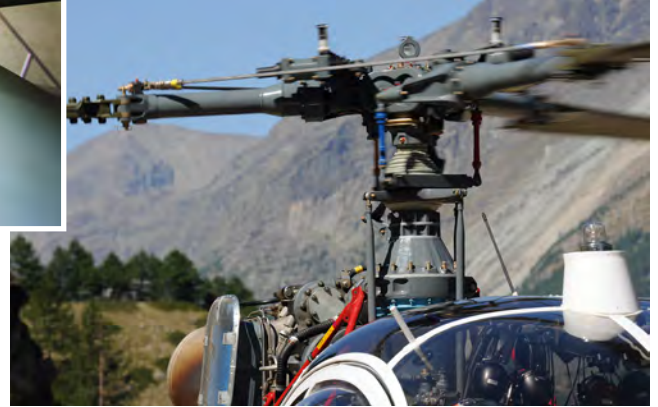
Above: A bad damper may produce a subtle transient vibration effect during turns.
