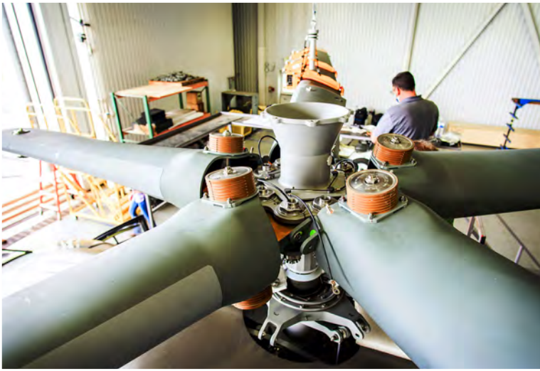
Left: Users found the track conditions of the rotor directly related to vibrations in the airframe.
