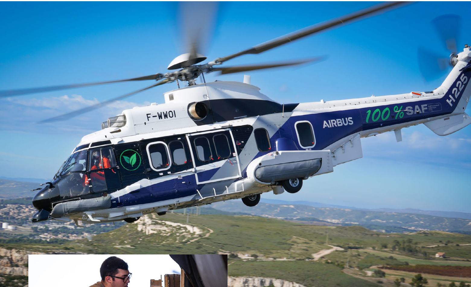
Above: The fundamental feature of a helicopter's design, a rotating wing, decouples the vehicle airspeed from that experienced by the airfoil or blade element on its main rotor.
