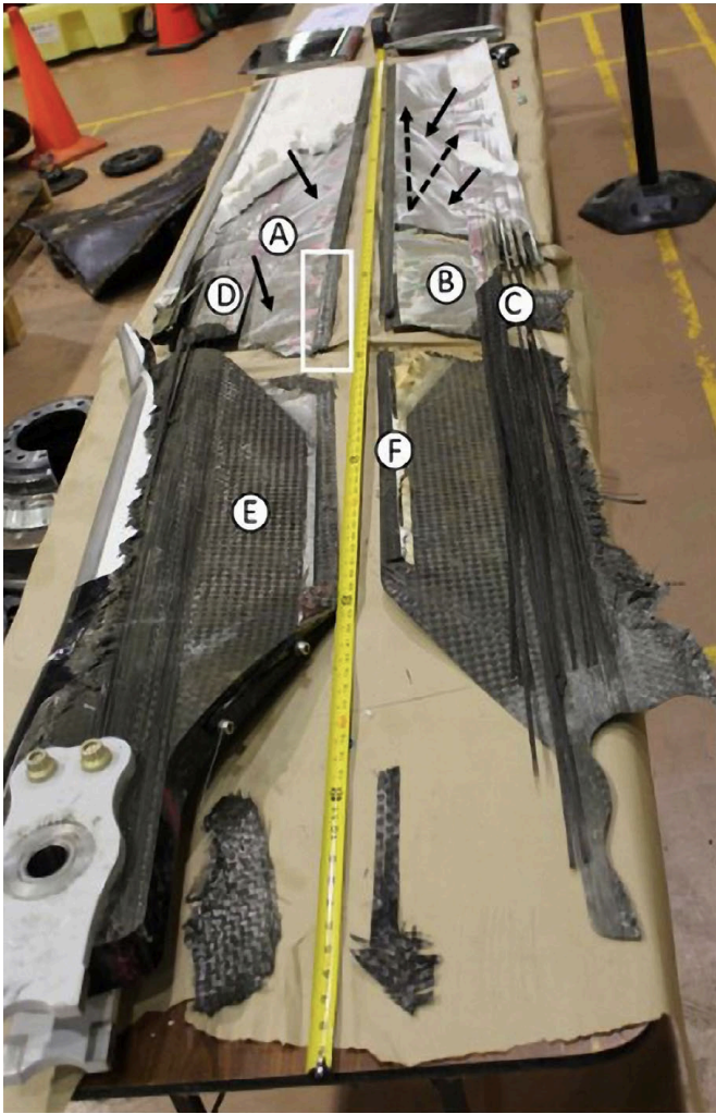
A -Lower skin B -Upper skin C -Upper spar D -Lower spar E -Upper filler ply stack F -Trailing edge strip Solid black arrows - symmetrical fracture arrest lines or tidal marks Dashed black arrows - direction of failure at station 60 White rectangle - area of discoloration on trailing edge strip
