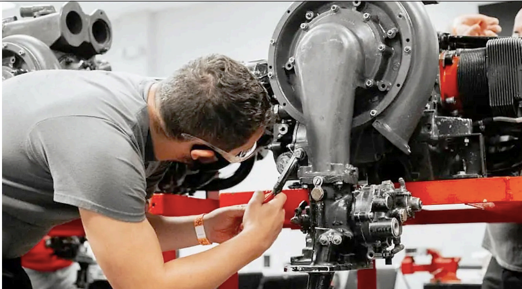
Above: Incorrect torquing or incomplete assembly of nuts, bolts, cutter pins, or safety wires accounts for a significant number of maintenance issues.
