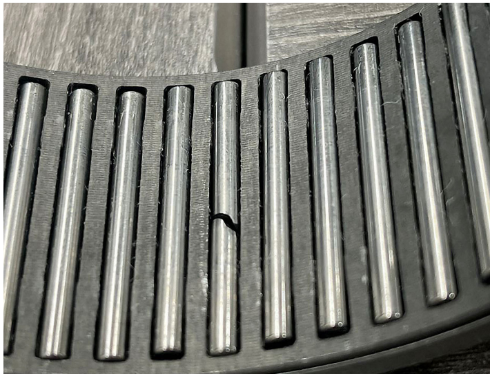
Below: Bell 505. Fractured roller in bearing.
