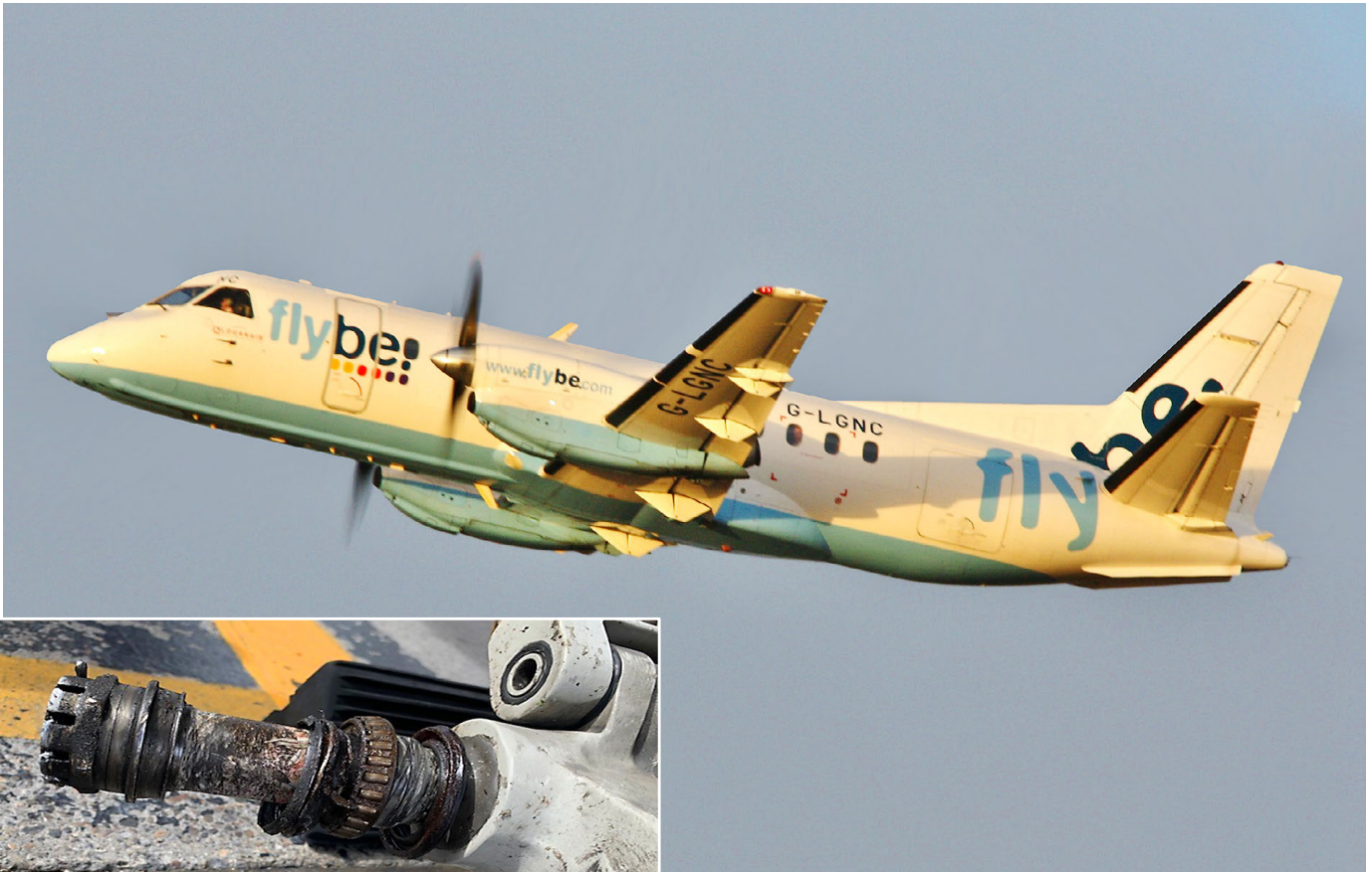
Above: A SAAB 340B in flight. Left: The axle with the remainder of the wheel bearings after the wheel departed the aircraft on takeoff.
