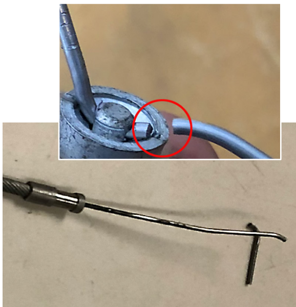
Bottom: Broken fuel selector valve control cable inner wire.
