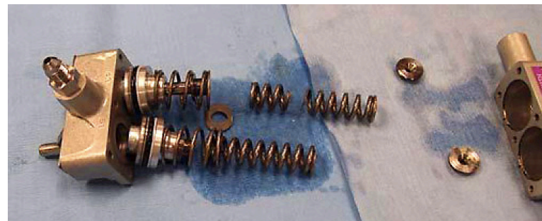
Above: Close up of a broken spring of the BCV.
