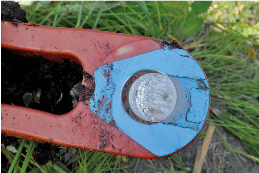
Above: Main rotor blade A strap and failed hub strap retaining pin. Above right: The occurrence helicopter's 4 main rotor hub strap retaining pins. Below left: The shipments of conforming pins (left) and non-conforming pins (right). Bottom: Map of the accident site and approximate fire area, with the accident site staging area in inset. Right: Example of 316 stainless steel pin on the left and H11 tool steel pin on the right. Bottom right: Shaded boxes denote the strap restraining pin (16) and the strap.
