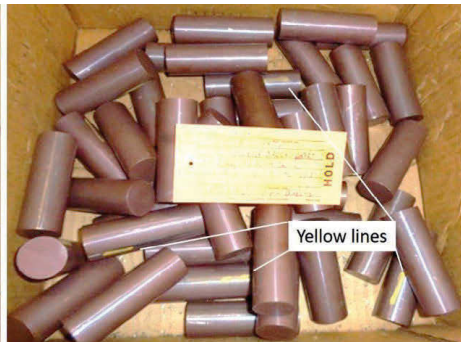
Above: Main rotor blade A strap and failed hub strap retaining pin. Above right: The occurrence helicopter's 4 main rotor hub strap retaining pins. Below left: The shipments of conforming pins (left) and non-conforming pins (right). Bottom: Map of the accident site and approximate fire area, with the accident site staging area in inset. Right: Example of 316 stainless steel pin on the left and H11 tool steel pin on the right. Bottom right: Shaded boxes denote the strap restraining pin (16) and the strap.
