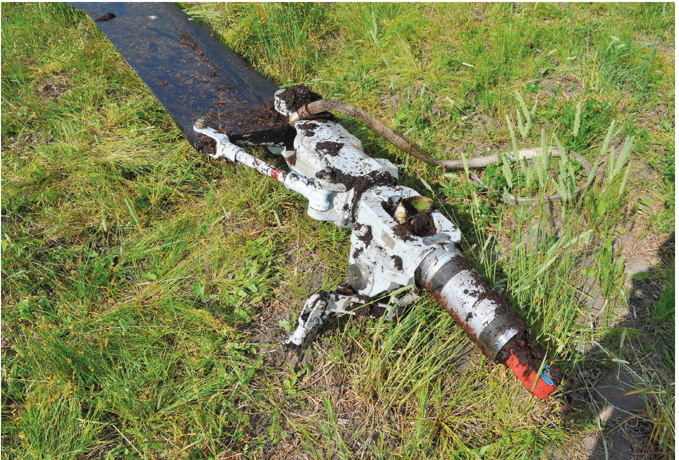
Above: Map showing the location of the staging area and accident site, with inset photos of the 2 main rotor blades. Below: Photo of the main rotor blade B and rotor head assembly.
