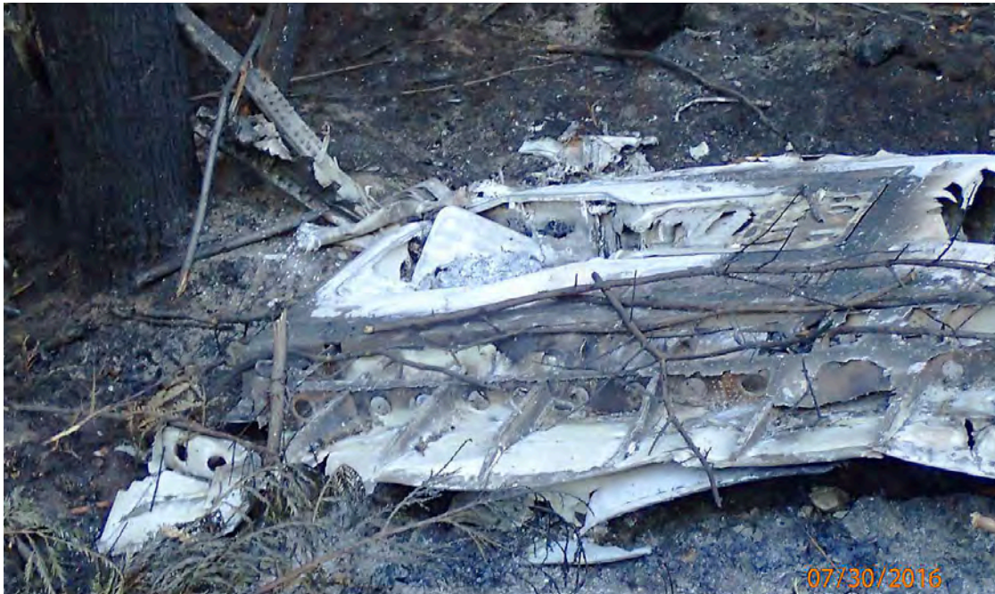
The left inboard wing section (above) at the accident site near McKinleyville, California (far right).
