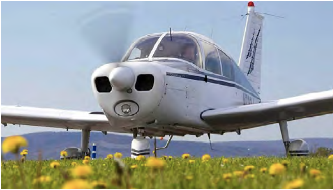
Piper Cherokee aircraft such as this have a Maximum Allowable Take-off Weight - 2,150 pounds.
