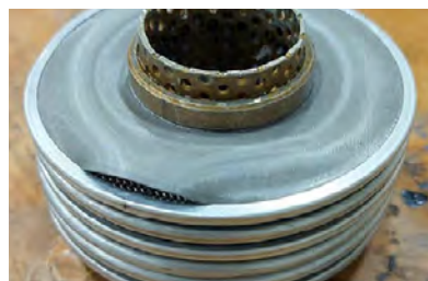
BEECH. (above) View from upper access panel with OUT marking evident. (left) Bulged filter disc due to the fuel flowing in the opposite direction than designed.
