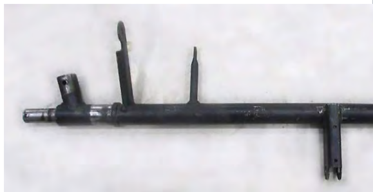
Report: CESSNA 150M Rudder Pedal Torque Tube Failure
