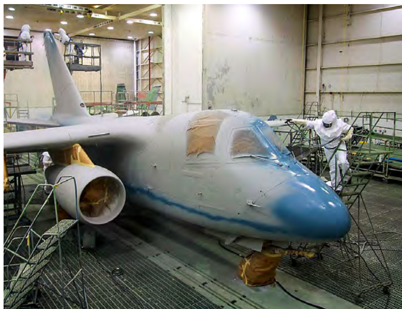
Aircraft painter applying an anti-corrosion formula.
