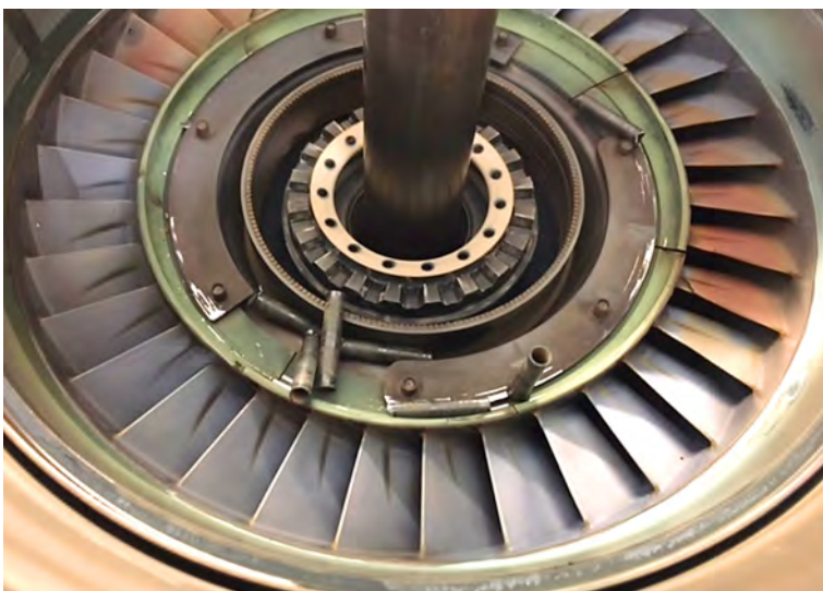
Honeywell. Rotor assembly with rivets that had fallen out due to incomplete setting.
