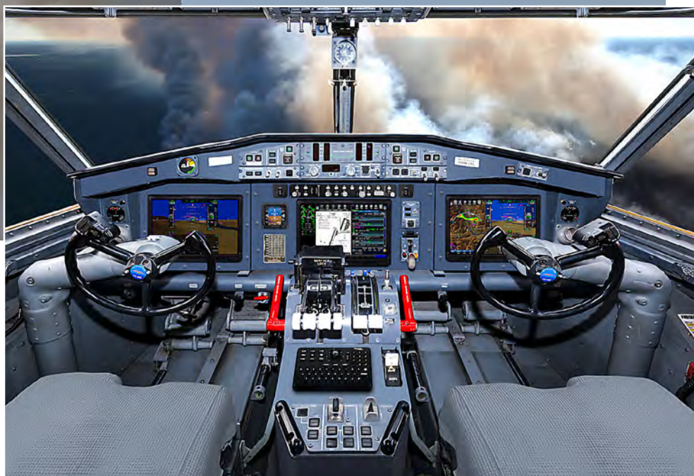
Right: The CL-515 integrates a Collins Pro Line Fusion digital avionics suite.
