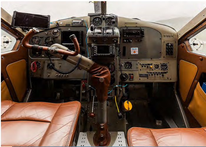
Left: The DHC-2 Beaver's single yoke can be handed over to the co-pilot, in flight
