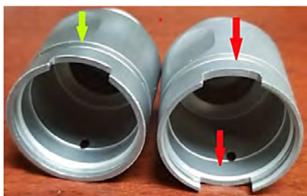
Above: Rolls-Royce. 1 and 2 slot-bearing-housing-assembly-configurations.
