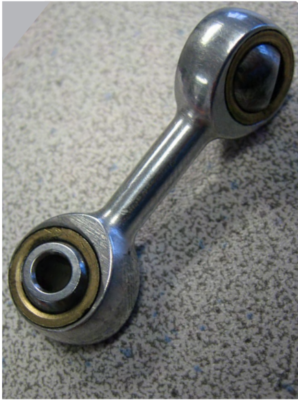
Pre R44 SB-71 throttle link P/N B564-2 having aluminum-bronze bearing races.
