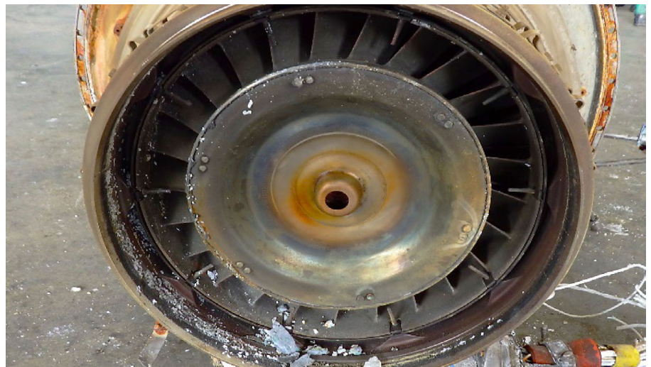
Above: Accident airplane's instrument panel. Right: Left engine power turbine vane ring. Bottom: Left engine propeller hub flange and beta ring.
