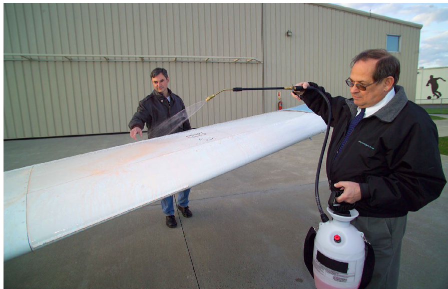
Below: Passive coating applications (below) that function synergistically with the active de-icing device is an attractive approach to de-icing.
