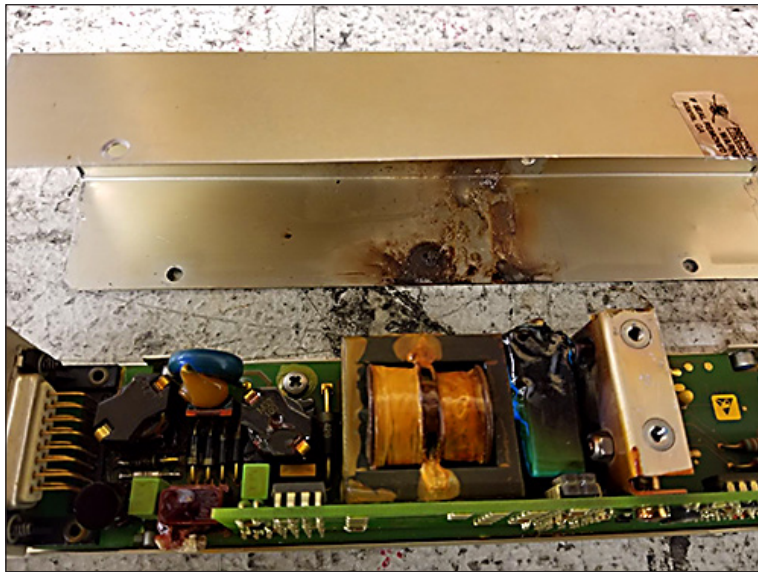
Dornier-Scorching and heat residue on the inside surface of the Ballast cover.
