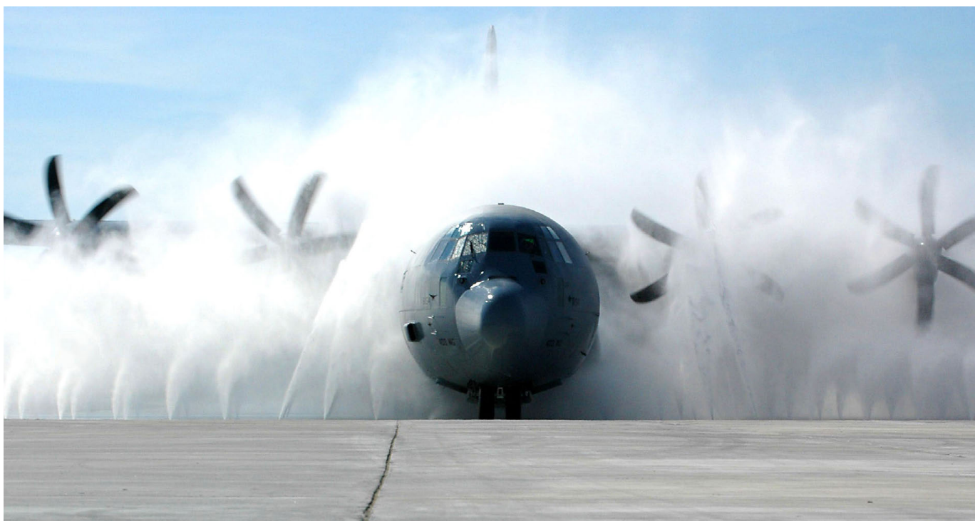
A C-130J Super Hercules is cleaned in the wash system.
