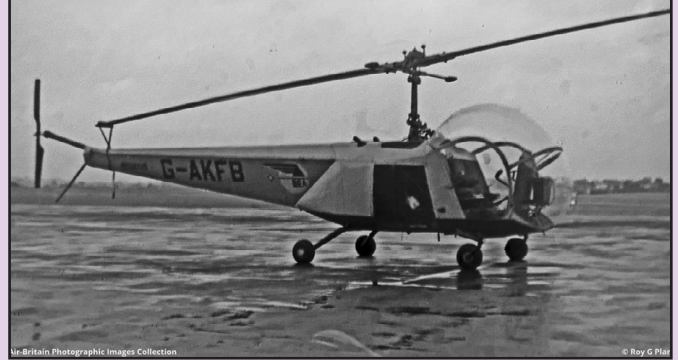
The Bell 47B has a quadricycle landing gear.
