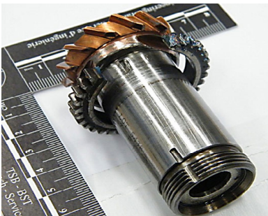
Top: C-FDKM in flight with birds deployed. Top right: Simplified schematic of the left wing fuel system. Bottom left: Gear which failed and was no longer keyed to the torque sensor shaft. Bottom right: Tooth wear on the loaded face and flank. Far right: No. 2 ejector nozzle and foreign object debris.
