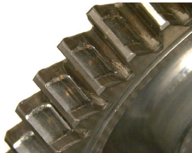
Top: C-FDKM in flight with birds deployed. Top right: Simplified schematic of the left wing fuel system. Bottom left: Gear which failed and was no longer keyed to the torque sensor shaft. Bottom right: Tooth wear on the loaded face and flank. Far right: No. 2 ejector nozzle and foreign object debris.
