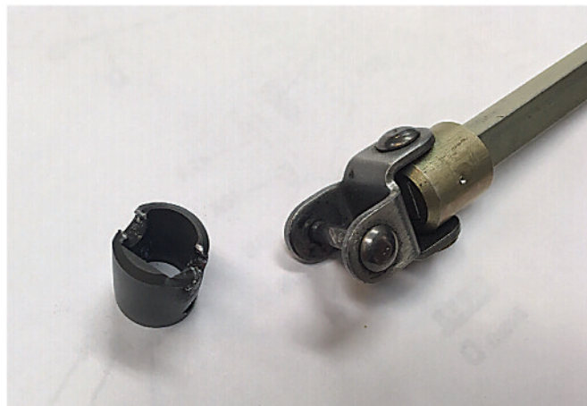
Above: Excessive wear resulting in drive shaft disconnect on a Cessna 172. Below left: A damaged battery from a Bombardier BD 700.
