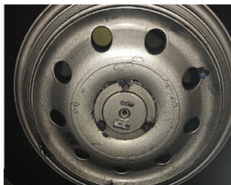
Left: Dassault Falcon. Wheel after being found. Bottom left: Axle showing bearings still there and wheel missing. Bottom right: Inside of wheel showing residual materials from broken bearing. Note the different sizes of bearing races with larger diameter inner bearing.
