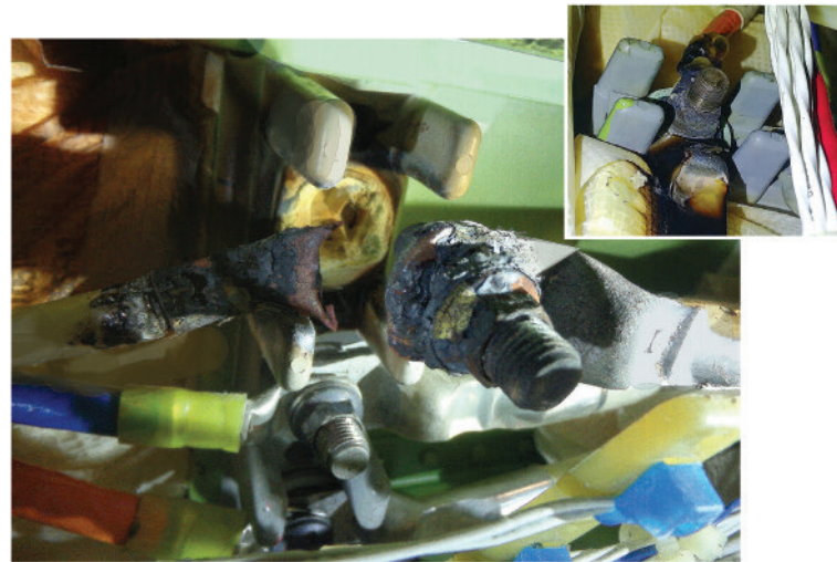
Above: Example of a B300 Cracked Aileron Weight on a Beech B300. Right: A Bombardier CL600's terminal block (TB33) burnt wires. Inset: Terminal block (TB18) burnt wires.
