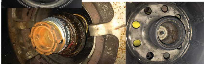
Left: Dassault Falcon. Wheel after being found. Bottom left: Axle showing bearings still there and wheel missing. Bottom right: Inside of wheel showing residual materials from broken bearing. Note the different sizes of bearing races with larger diameter inner bearing.
