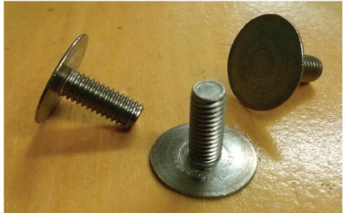
Above: Click Bond fasteners made from 300 Series Crest Stainless Steel ( capable of 500 lbs. of pull and 1200 lbs. of shear ) for mounting canard ailerons and rudders. Below: A jumble of specialty drilled fasteners and skin fasteners for interior and airframe applications.
