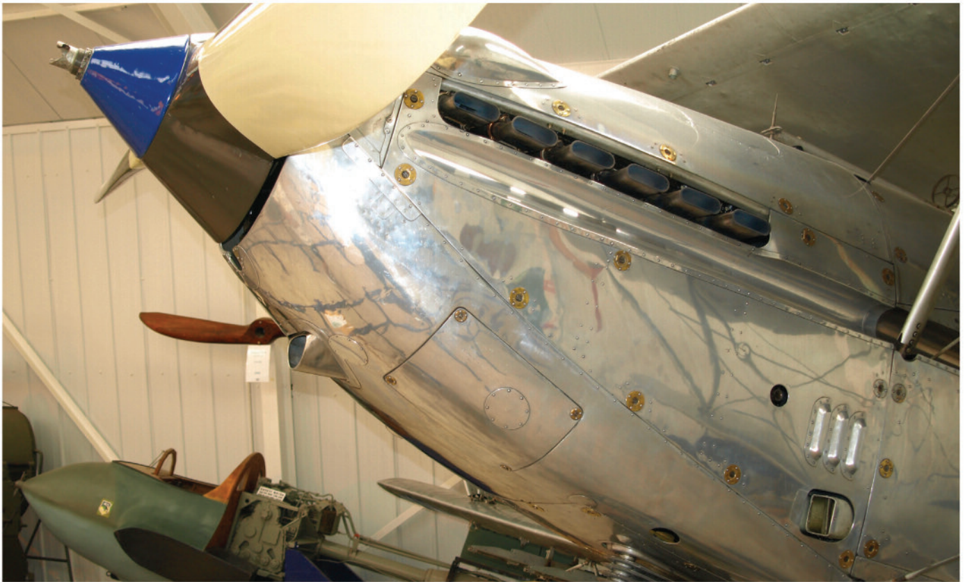
Dzus fasteners attach the cowling panels of the 1930s Hawker Hind.
