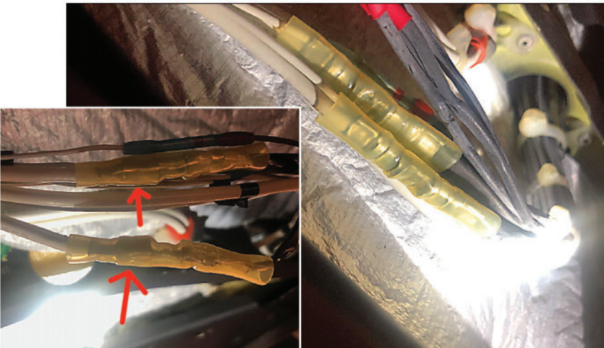
Above: Properly spliced wiring versus improperly spliced wiring (inset).
