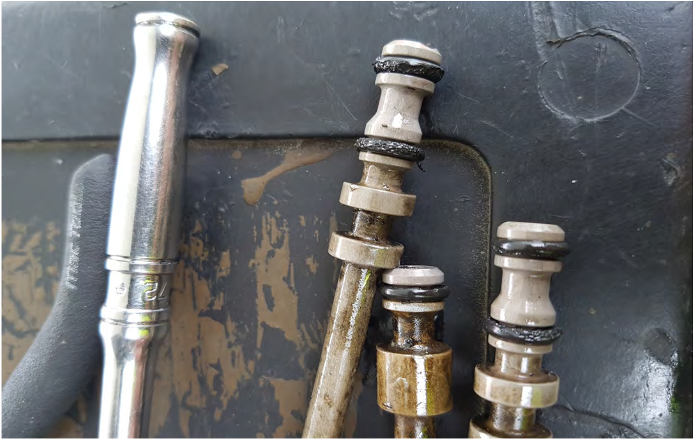
Above: Pratt & Whitney. Fuel tubes with Skydrol damaged O-rings.
