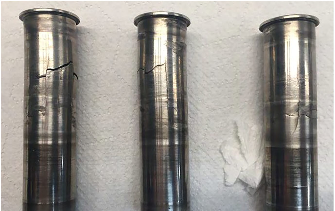
Above: General Electric. Damaged fan blade retaining pins.
