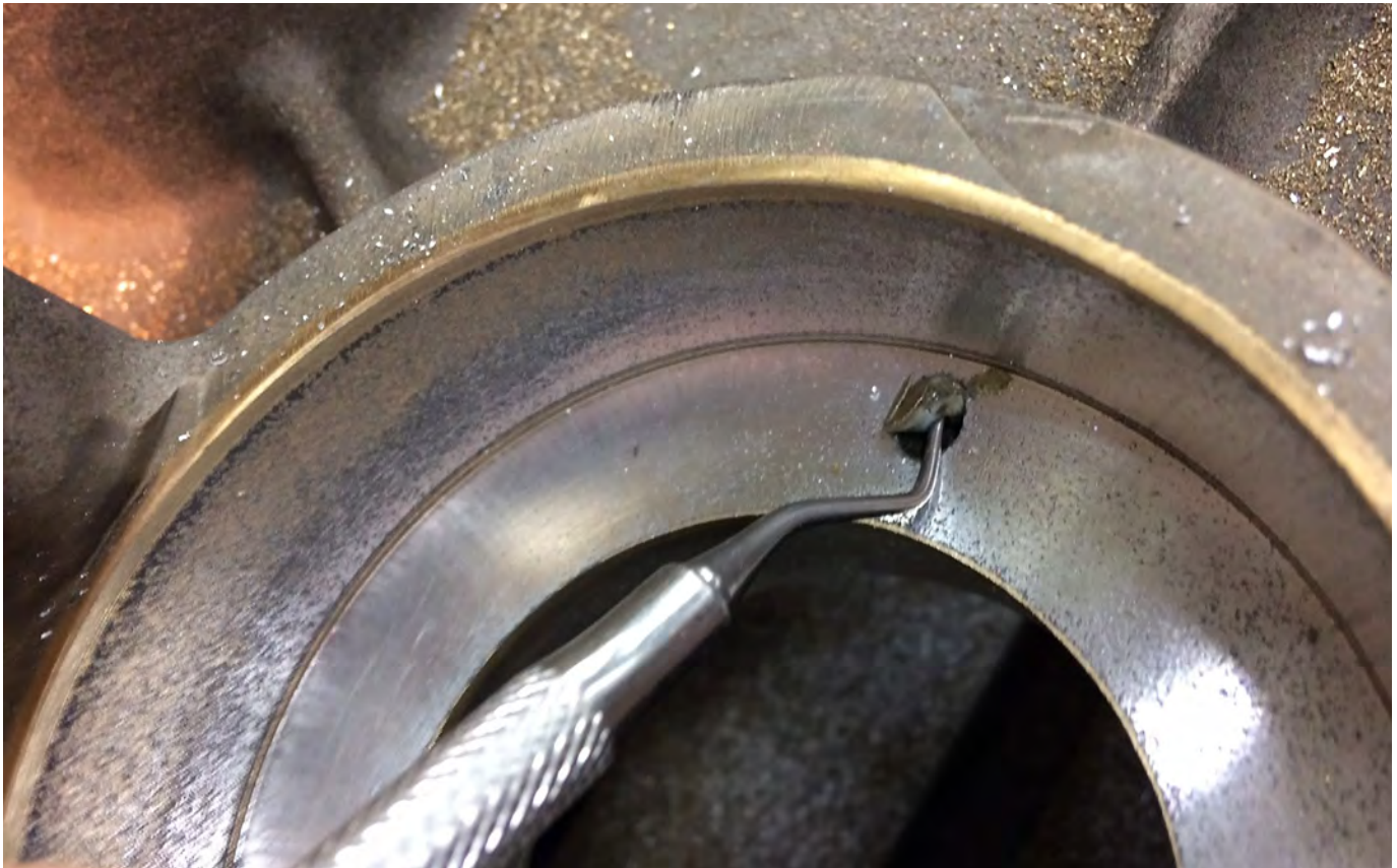
Above: Rolls-Royce. Bearing cavity with rubber plug left after previous repair.
