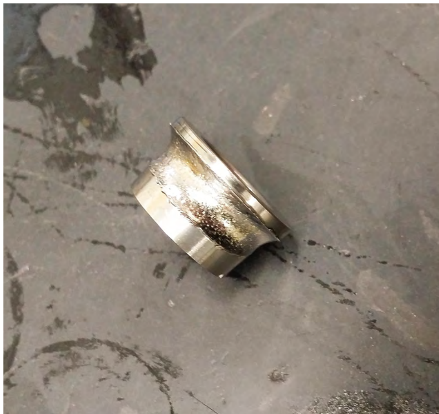
Above: Garrett. Engine SOAP Sample. Idler bearing race showing significant wear.
