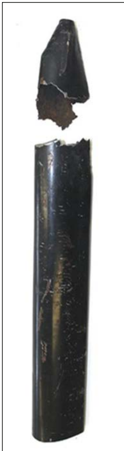
Left: Damage on the upper half of the left main spar wing lift strut assembly. Above: Result of the failed wing lift strut assembly.
