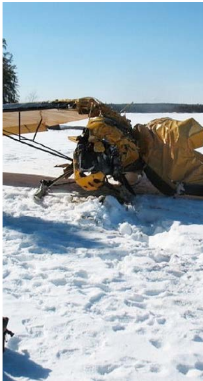
Left: Damage on the upper half of the left main spar wing lift strut assembly. Above: Result of the failed wing lift strut assembly.
