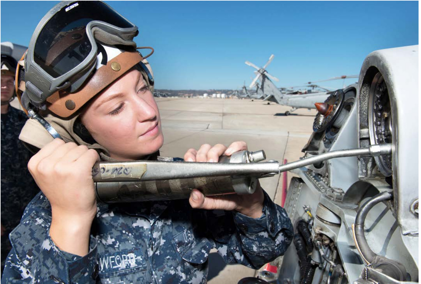
Above: Humidity, atmospheric pressure and the amount of salt and dust an aircraft is exposed to determine which grease to use.
