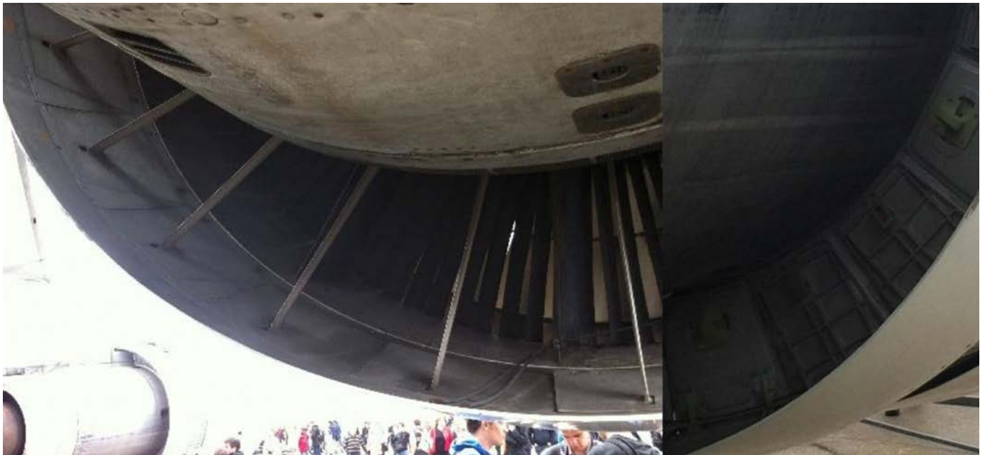
Above: The TRAS, seen here stowed and deployed on a 747, blocks bypass air from exiting the engine to the rear during landing.
