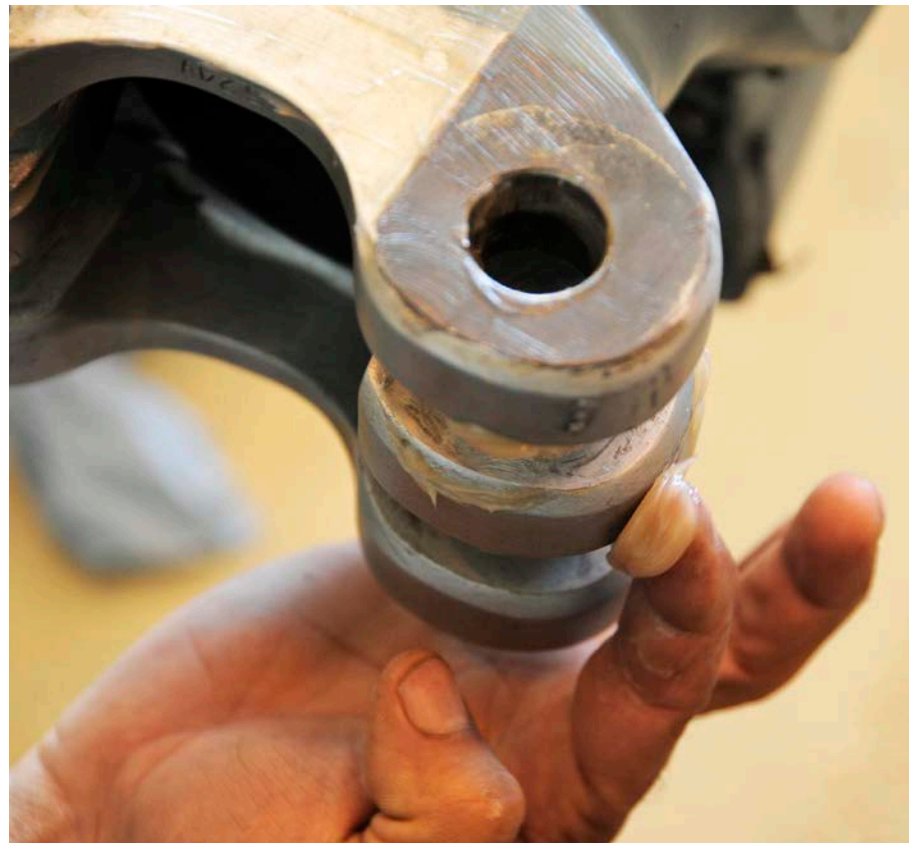
Above: An AME applies grease to the rotor blade of a helicopter.
