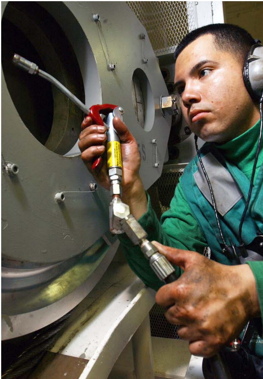
Above: Compared to other lubricants, greases are unique as they stay where they are put, act as a seal against dirt, dust and water.
