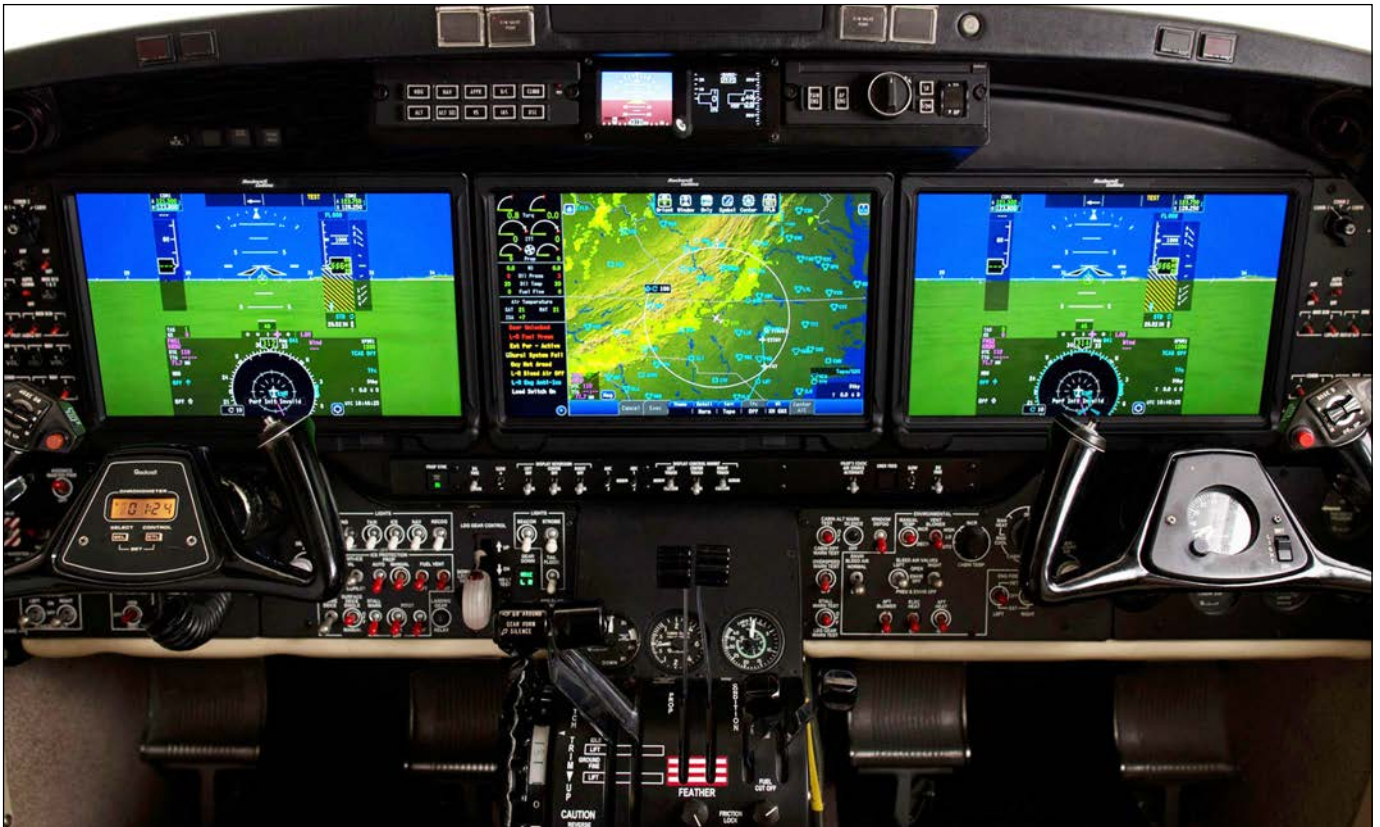
Above: Having an upgraded cockpit such as Primus Elite that includes ADS-B compliant transponders, GPS position sourcing and wiring eliminates the challenge of complying with ADS-B and other upcoming mandates.
