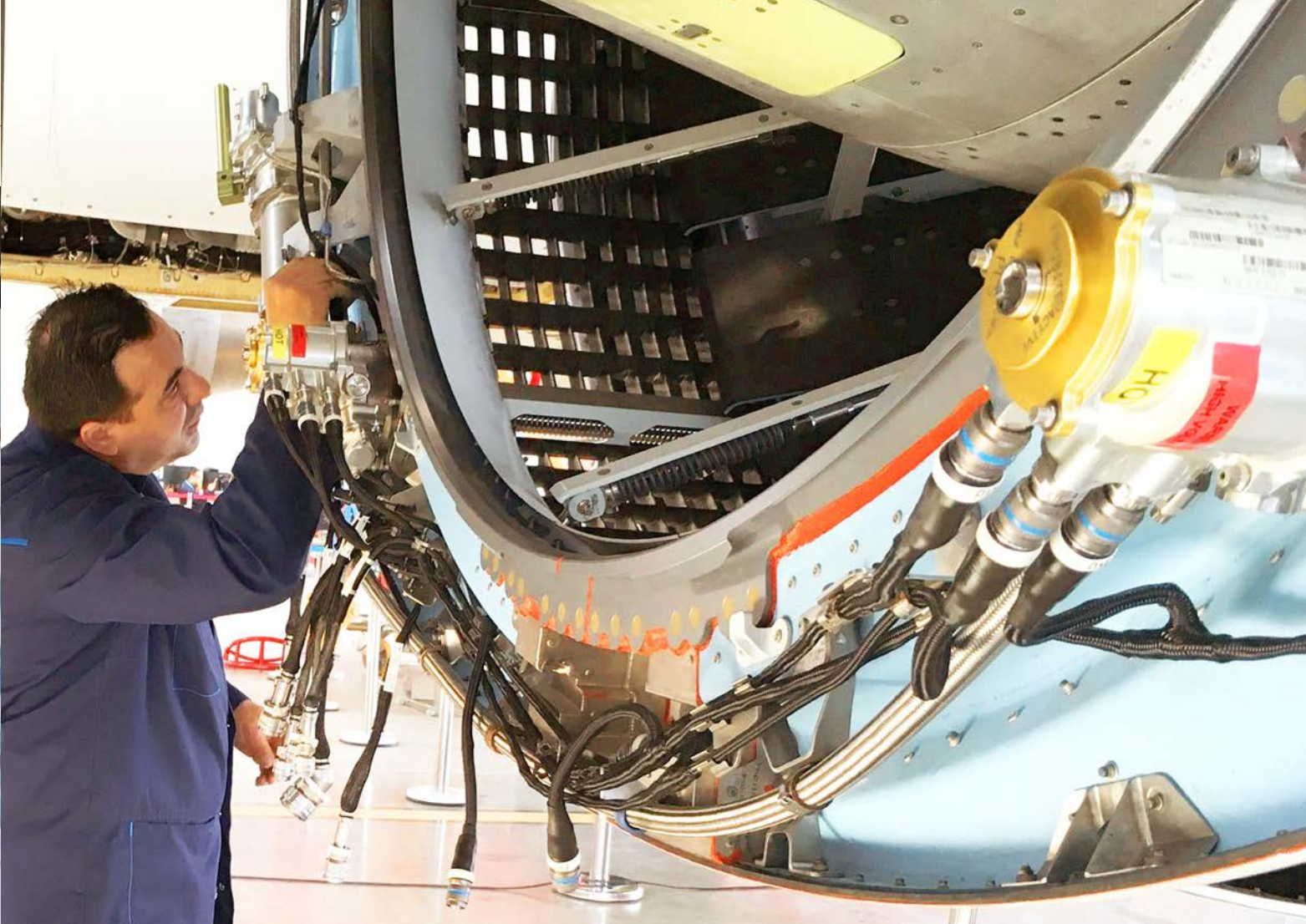
Opposite: During thrust reversal, flexible shafts translate the aft cowl to the rear to reveal a matrix of openings through which the bypass air is redirected. When deployed, actuators redirect bypass air through a mid-engine matrix. Above: The CFM International LEAP-1C includes Nexcell's O-Duct thrust reverser system.
