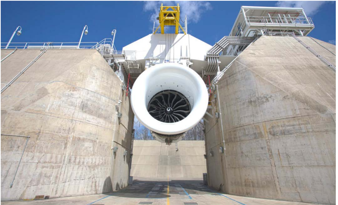
Above: At roughly 11 feet in diameter the giant fan is the GE9X's most distinctive feature.
