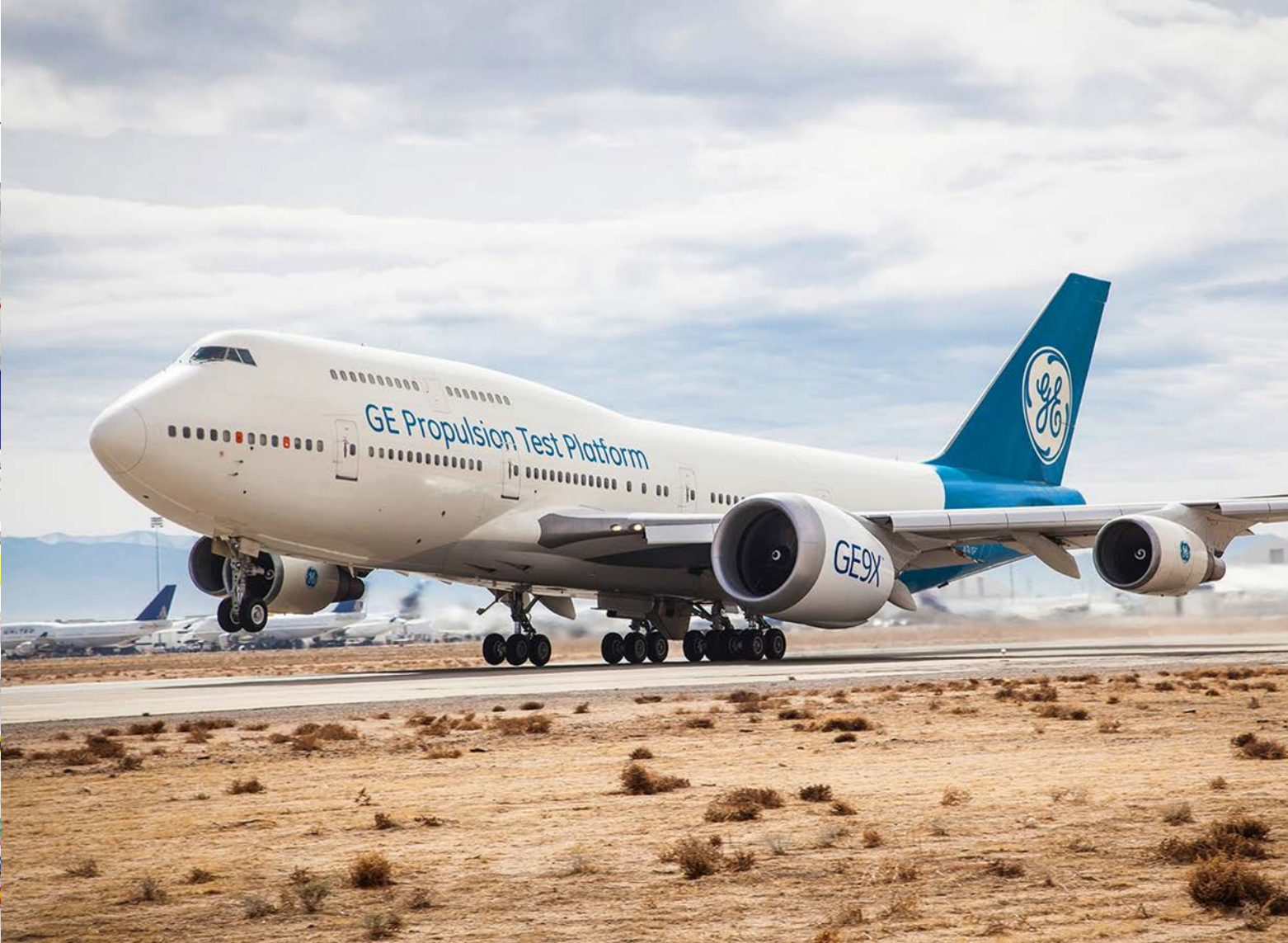
Opposite: GE90 engine. Above: “Mounting an engine of this size to our 747-400 is a challenge,” Jon Ohman says. “The engine is mounted on a unique pylon that cantilevers the engine out in front of the wing and tilts it upward by approximately seven degrees.”
