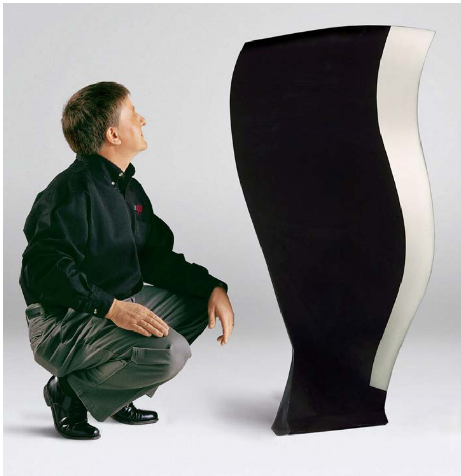
Above: The GE90 blade made its way to New York's Museum of Modern Art. Where the GE90 has 22 fan blades, the GE9X will have just 16 blades made from 4th-generation carbon fibre composite.
