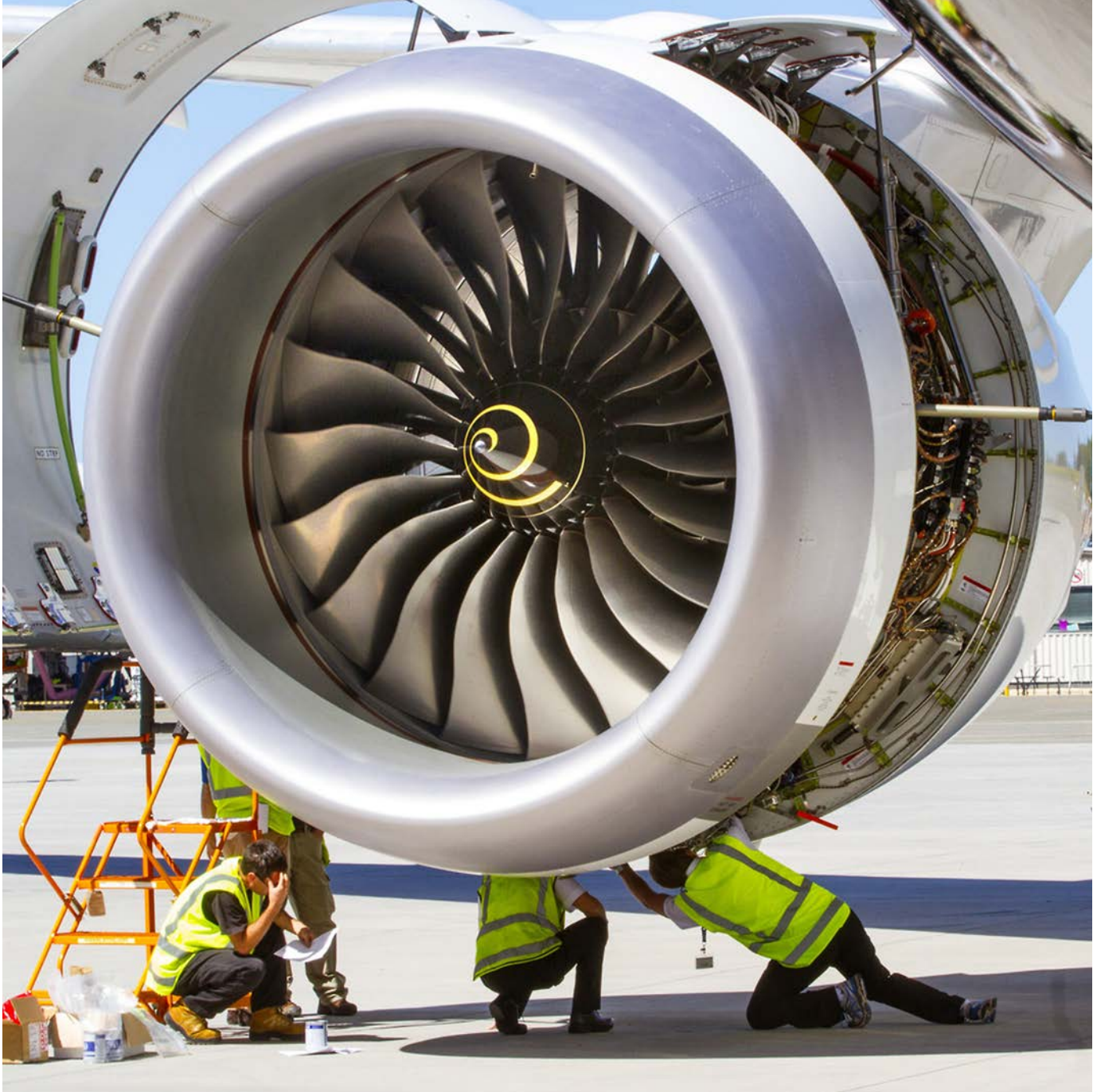
Above: Technicians make adjustments to a Rolls-Royce Trent 1000 engine on an Air New Zealand.
