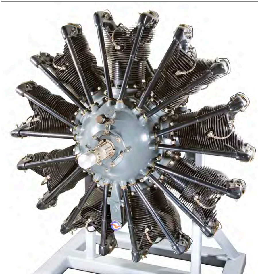
Above: P&W manufactured the R1340-series engine between 1925 and 1960. It has a history of cylinder failures.
