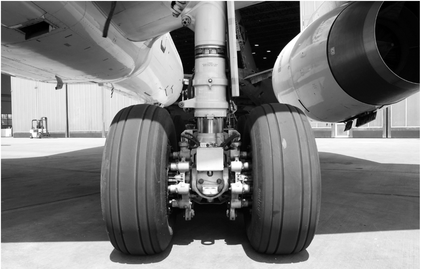
Above: Chrome has been long prized for its hardness and ability to minimize sliding wear on many applications such as landing gear.
