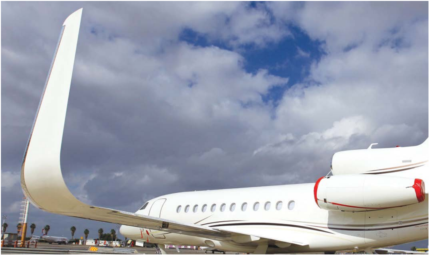
Above: This Falcon 900 features a blended winglet, which has a large radius and is designed with a smooth chord variation in the transition area where the wing joins the winglet.
