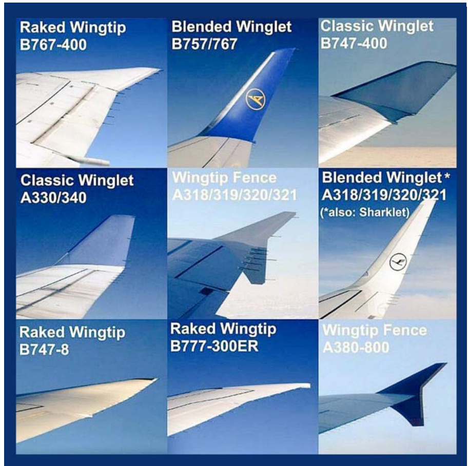
Photo right: Various aircraft winglet types.
