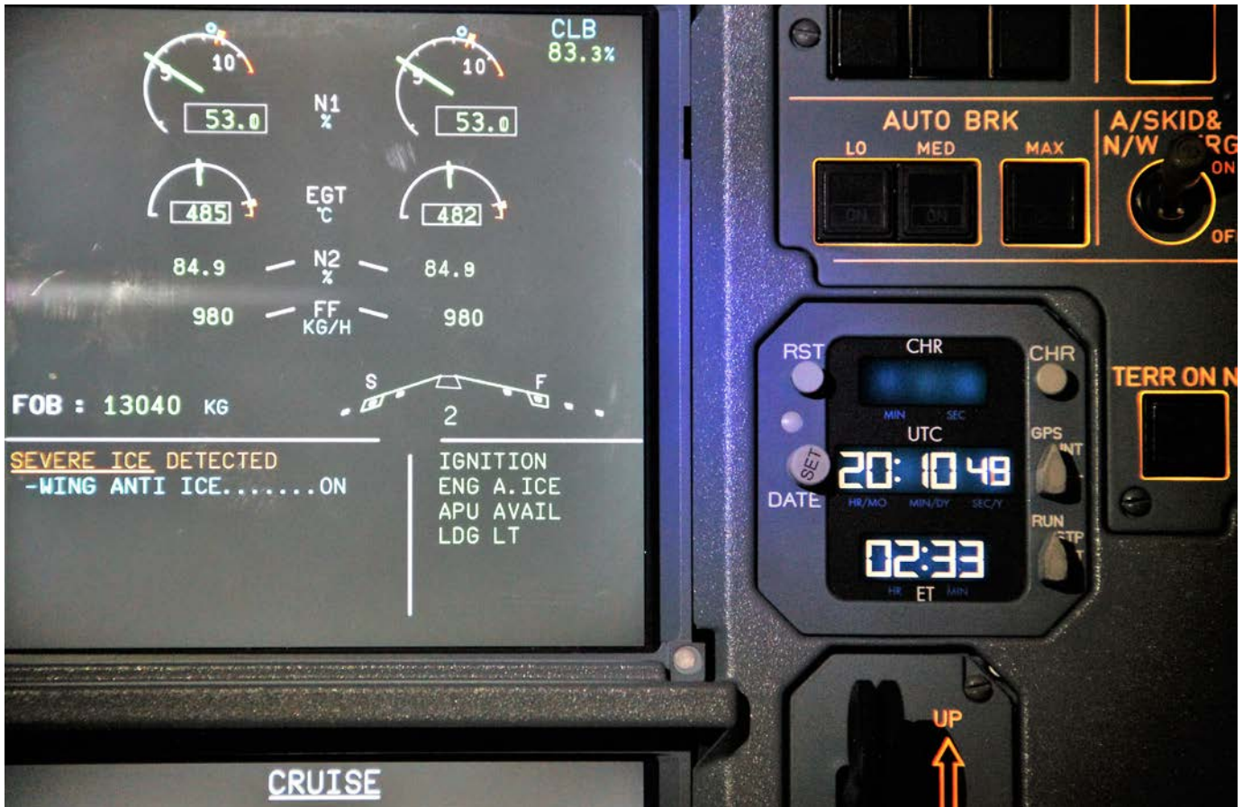
Above: Dual Advisory Ice Detection System. Severe ice detected on ECAM display.
