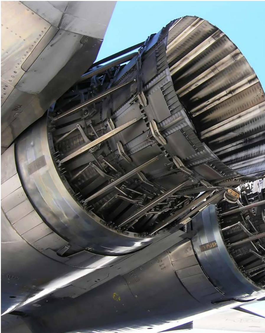
Above: A jet afterburner up close. Flex shafts drive the actuators that open and close it.
