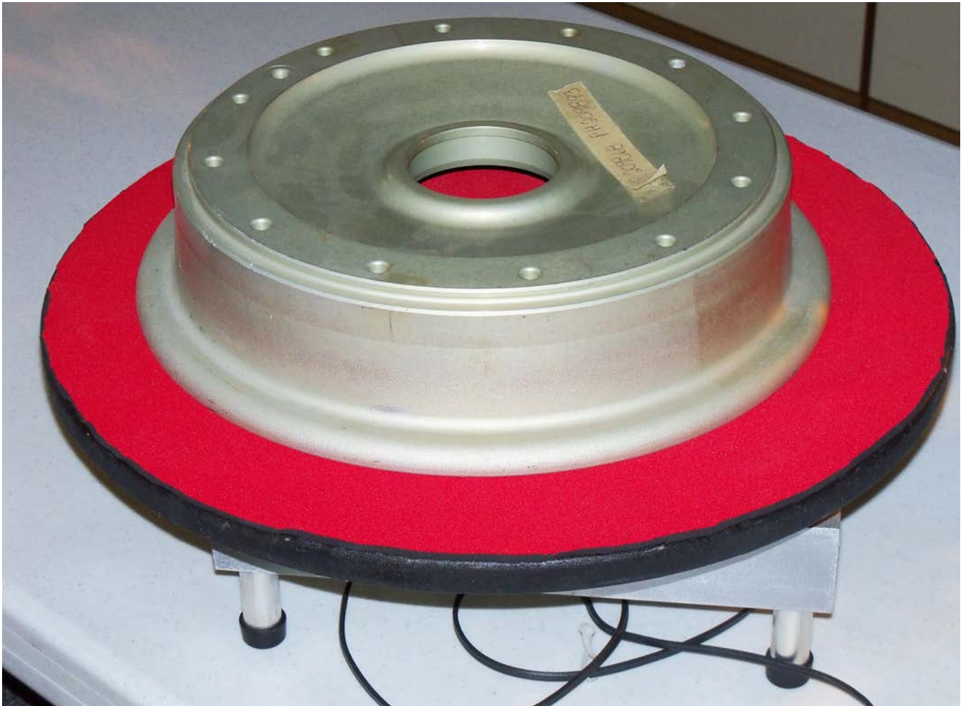
Above: Inspecting a wheel on a motorized turntable.
