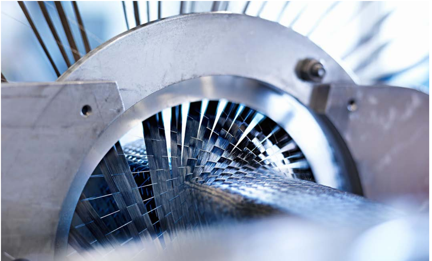
Above: Used extensively in the Airbus 350 XWB family, carbon-fibre reinforced plastic is lighter than aluminum and stronger than iron.
