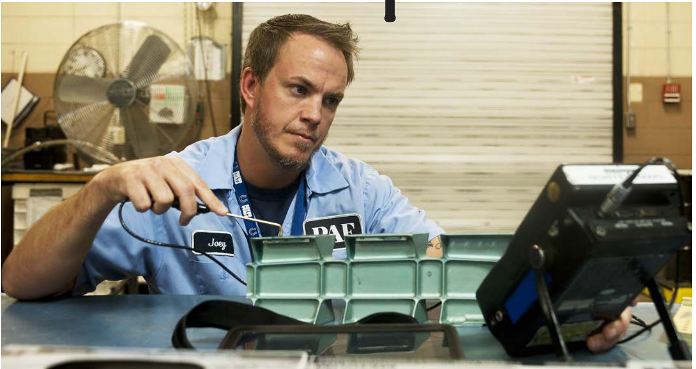
Above: This tech is looking for abnormalities and cracks on and around an aircraft part using an eddy current.
