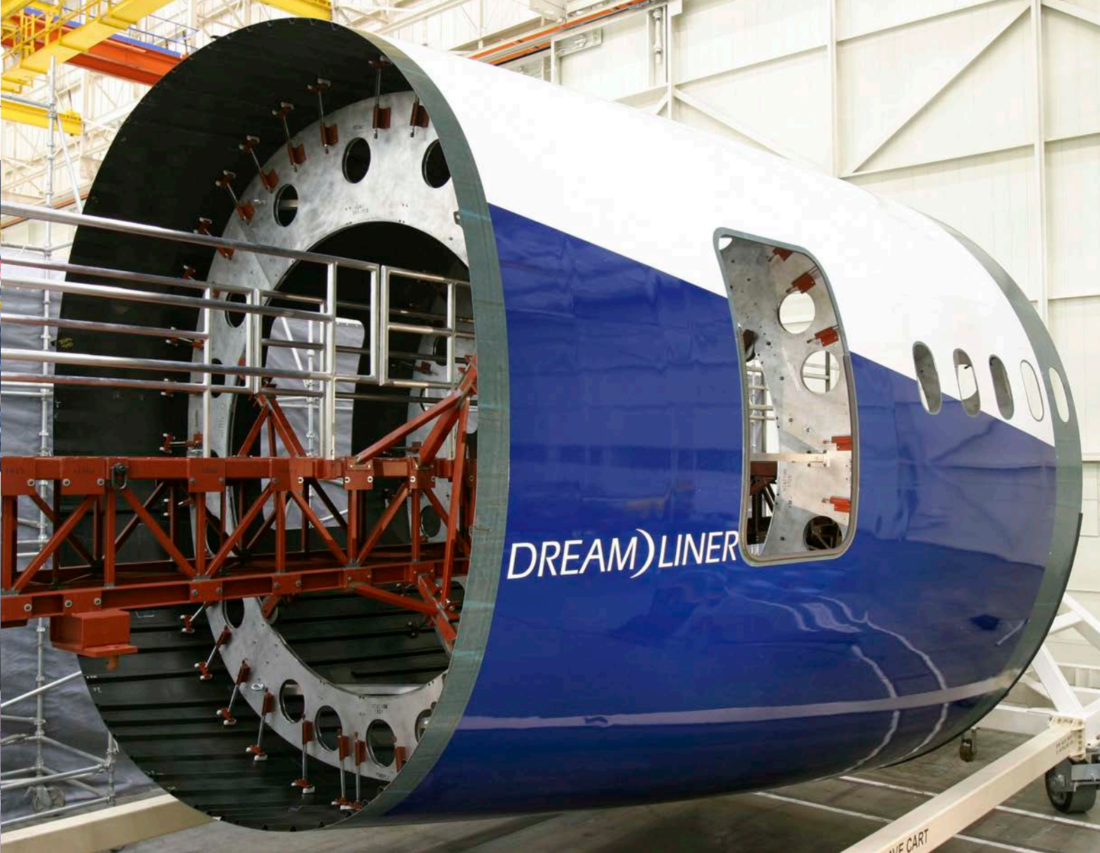
Opposite: A component of the Airbus A310 is fed through a high-tech loom where strands of carbon fibre are braided together. Above: By building the composite fuselage sections as full barrels with integrated stringers, Boeing reduced the number of parts on the 787, improving overall aerodynamic performance.
