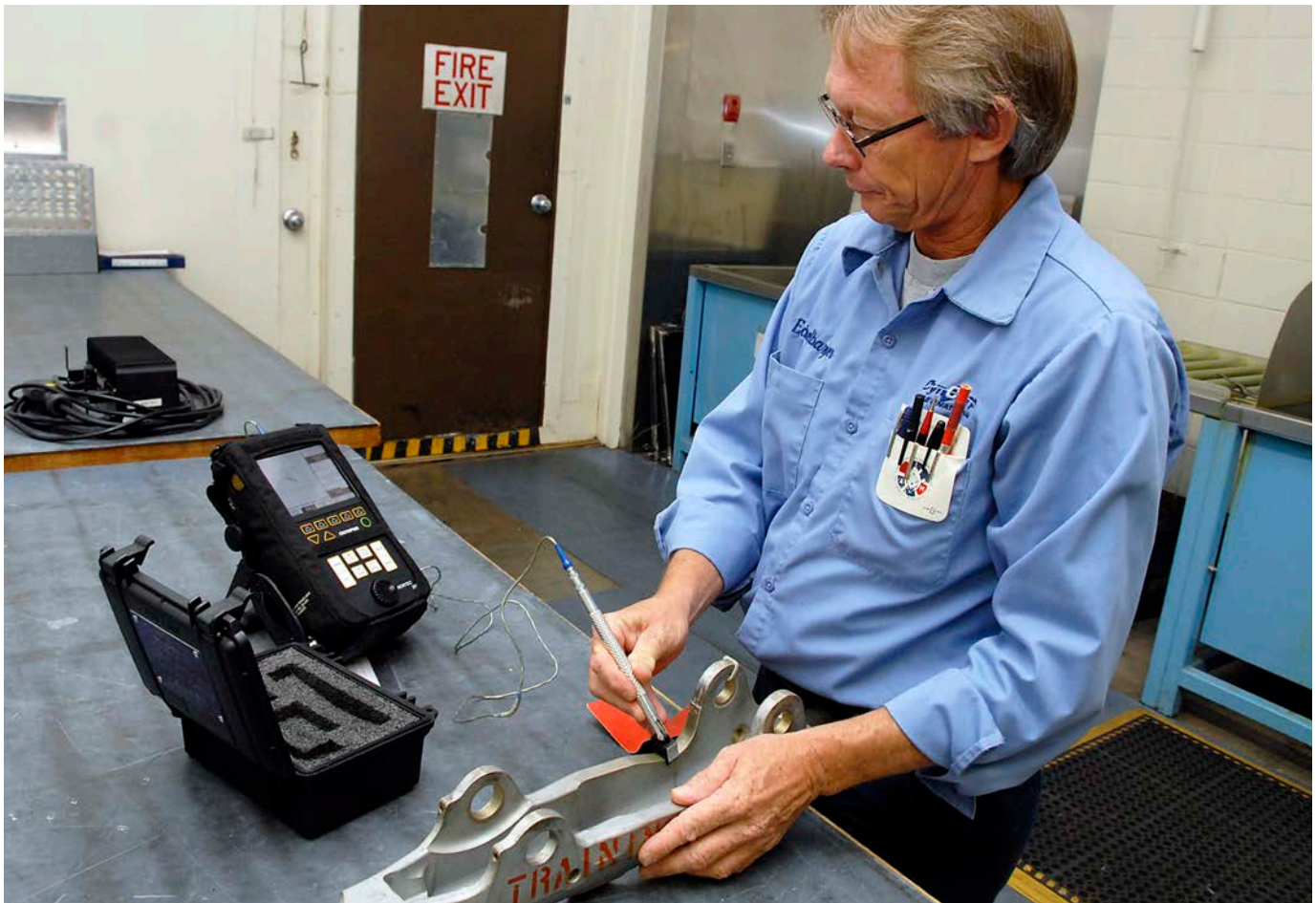
Above: A specialist at a non-destructive inspection shop uses an eddy current to search for defects in an aircraft part. An eddy current is the outer ring of a magnetic current
