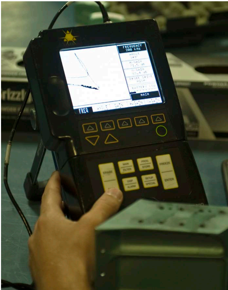
Above: Eddy testing has found a crack inside an aircraft part. An eddy is an electric current in a conducting material that can show cracks unseen to the human eye.
