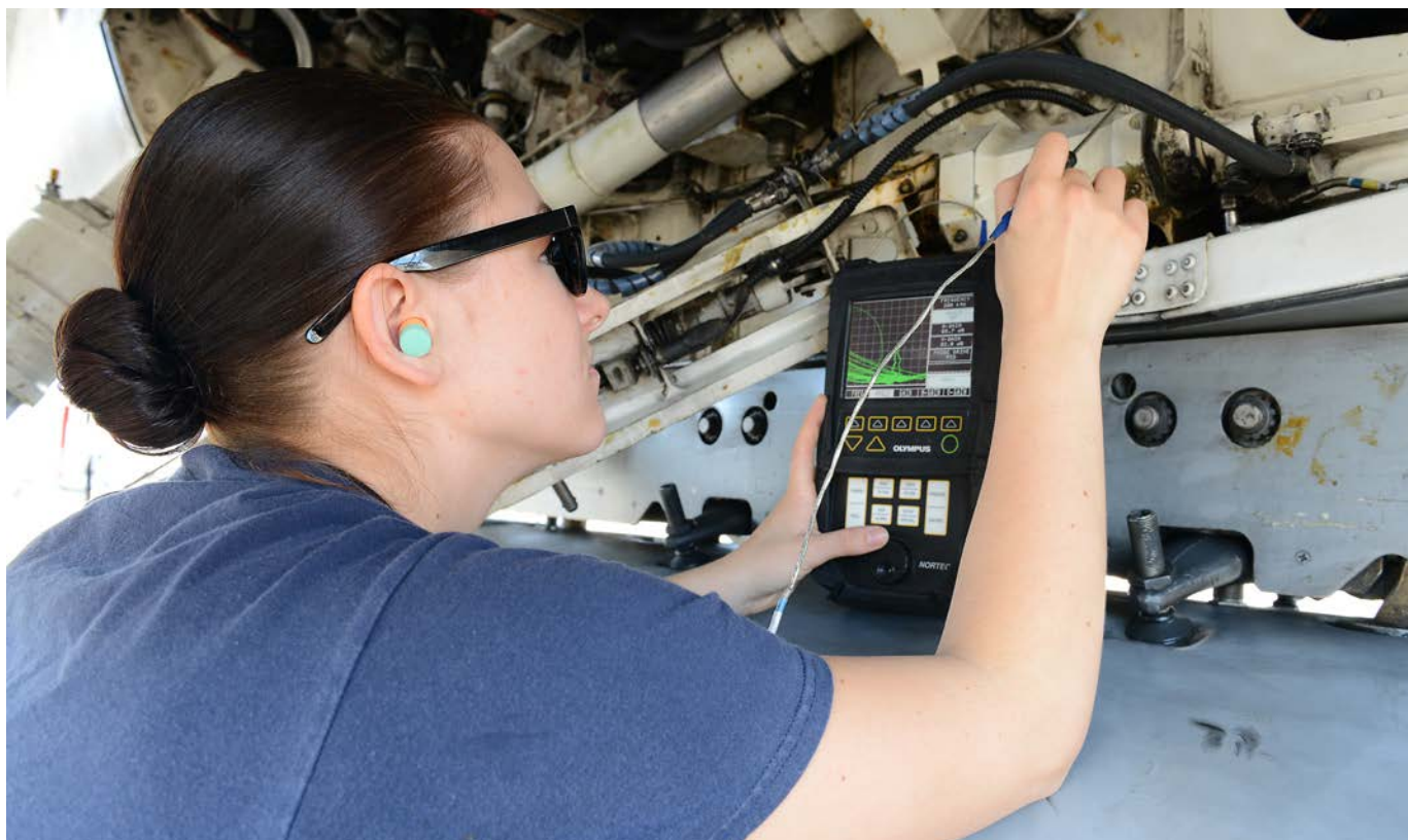
Above: This nondestructive inspection technician is performing an eddy current test to check for problems that may compromise the aircraft's structural integrity.
