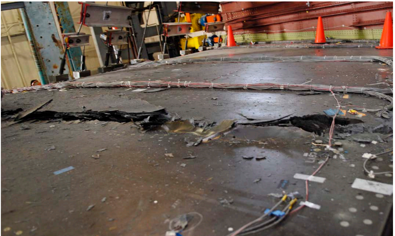
Above: Boeing Composite Manufacturing Center begins fabricating 787 vertical fin. Below: Boeing performs destructive testing on a full-scale composite wing box of the 787 Dreamliner, the first Boeing all-composite wing box ever built.
