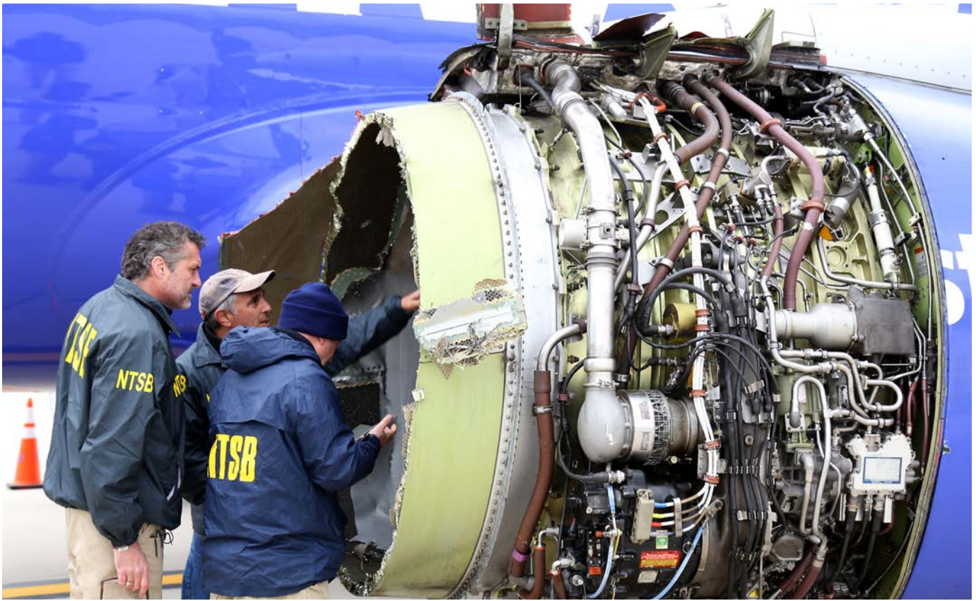
Above: NTSB investigators examine damage to the CFM International 56-7B turbofan engine belonging Southwest Airlines Flight 1380.
