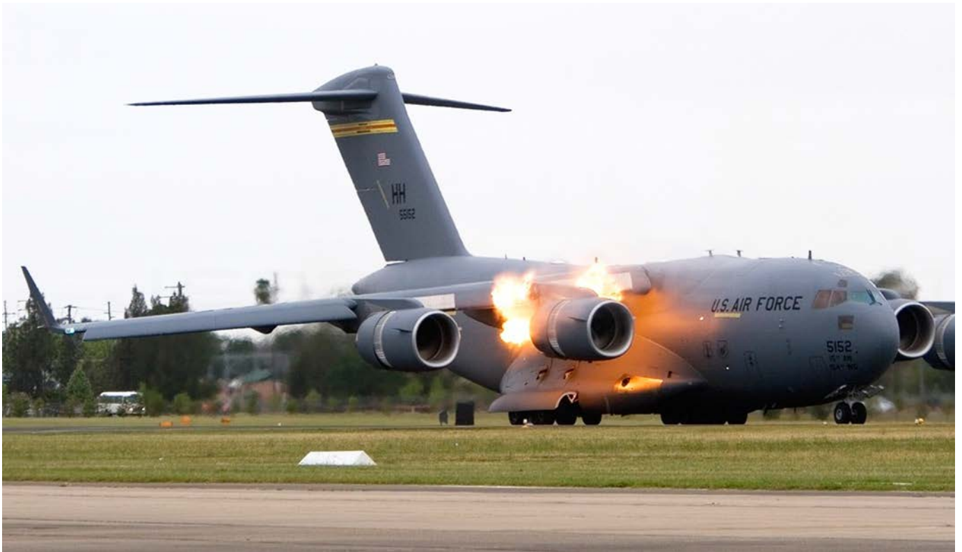
Above: A C-17 with an engine compressor stall during reverse engine operations. Below: An engine's compressor section.
