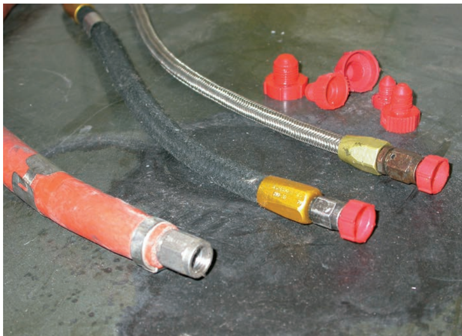
Engine hoses should be inspected for condition, time in service and be capped to prevent contamination.
