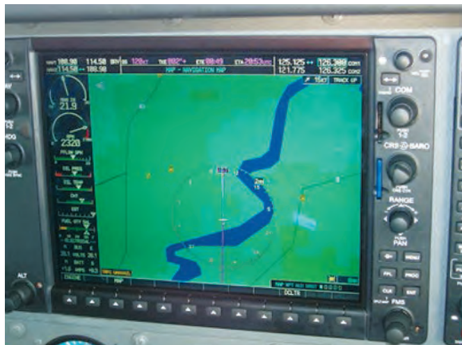
Many instrument-capable general aviation aircraft have GPS receivers and moving map displays.
