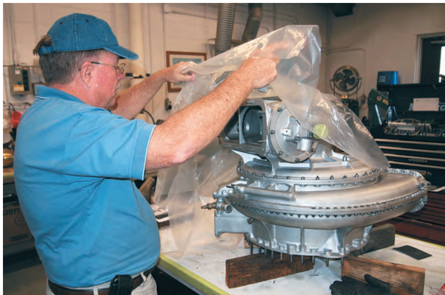
Bill Tate uncovers one of the North Star’s restored Merlin superchargers.
